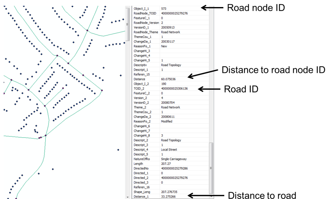
Figure 13-11 Data matching each building with the adjacent road, nearest node and the distances
