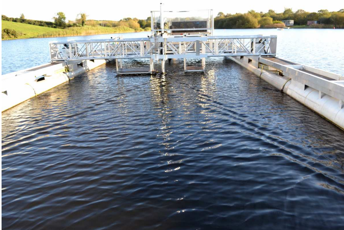
Figure 7: Twin hulls, surveying instrumentation support structure (stretching between and supported by both hulls) and wheel house of existing SuperGen Marine Allycat structure
