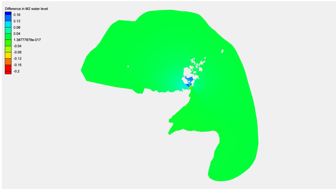
Figure 32 Difference in M 2 water level between natural case and a case with 3 rows of turbines
