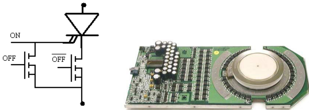
Fig. B3: 4.5kV ETO module with 4kA snubberless switching capacity.
