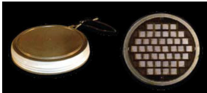
Fig. B4: Example of press-pack IGBT modules. (Source TMGE website).
