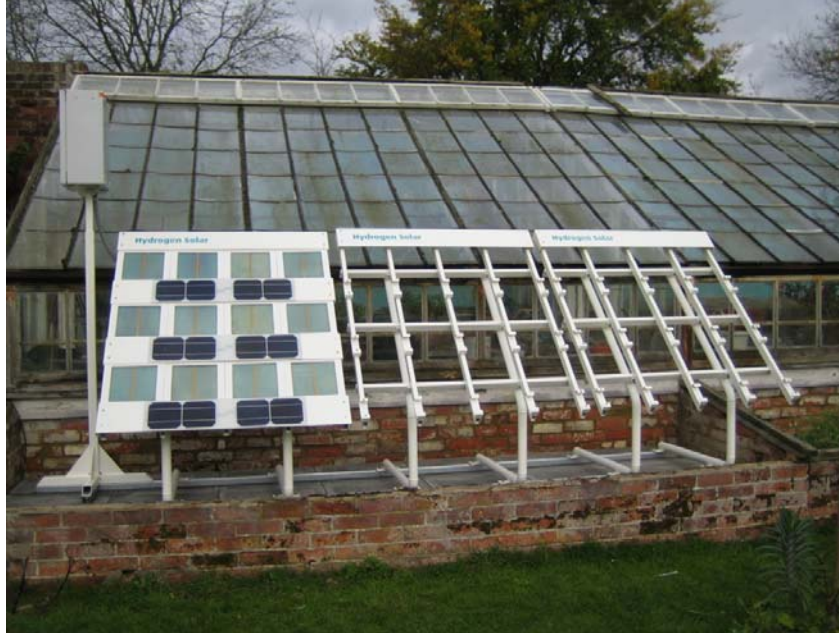
Figure 13 – 12 Cell array assembled at UK outdoor demonstrator site (a) Frame assembly constructed for three 12 cell modules
