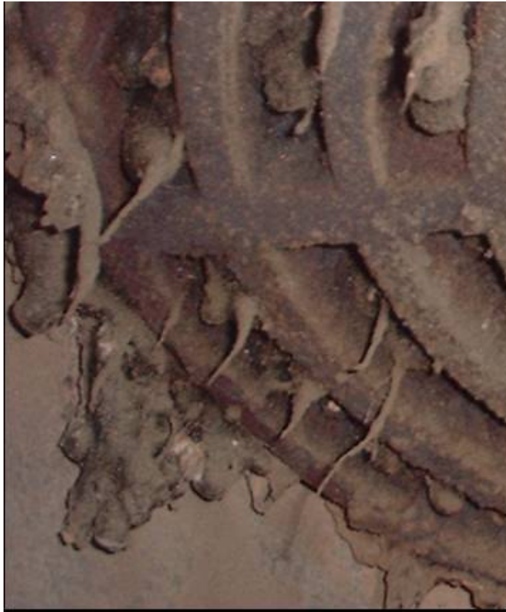
Photograph 6. Clinker/melt formation with RBF
