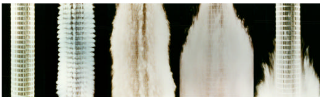
Figure 26. High Speed Photography Showing the Action of Pulsed Jet Cleaning. (Moving across the photograph from left to right: the metal fibre element loaded with dust; the dust is removed from the surface by the pulsed jet action; the dust is carried away; the dust begins to settle; and quickly falls to the bottom of the vessel leaving a clean element. Sequence time - half a second.)
