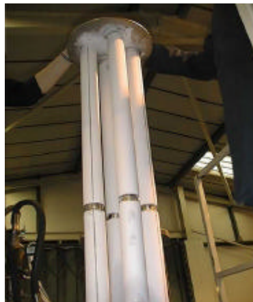
Figure 28. Testing of Filter Elements Using Dust Feeder Connected to Test Rig.
