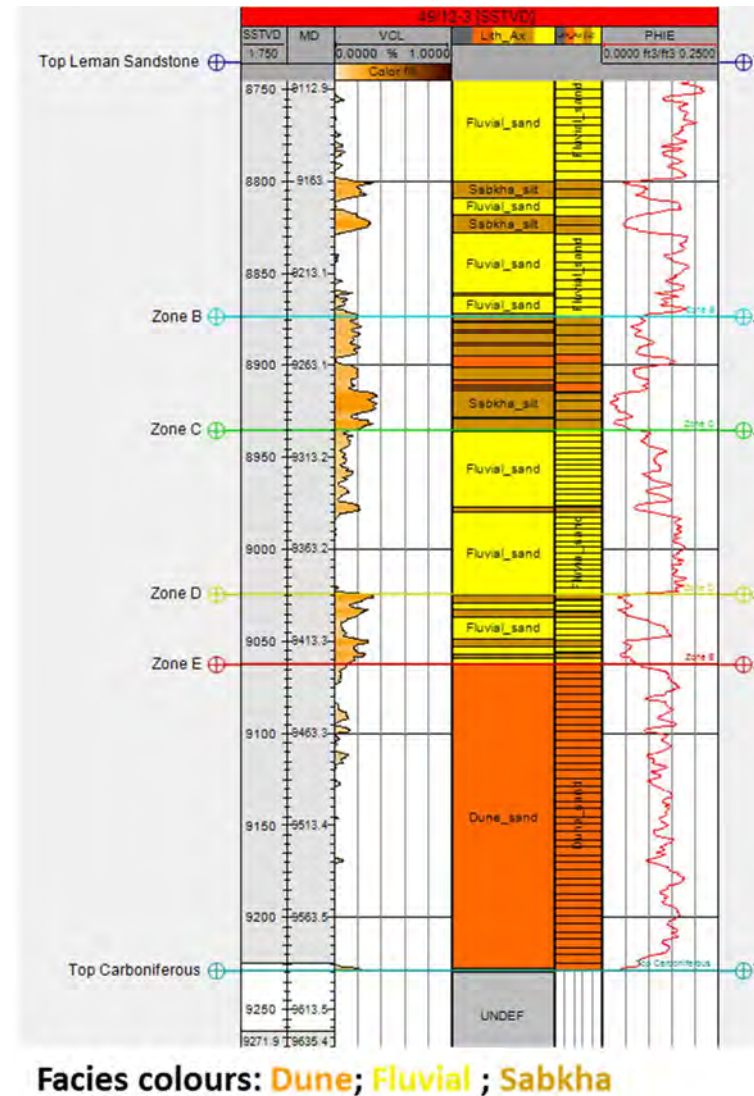
Figure 3-37 Example of facies interpretation in well 49/12-3
