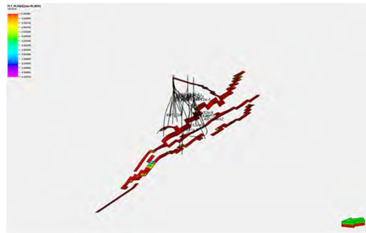
Figure 11-115 Fault cells (plastic shear strain property) at K layer 58 in the Lemman sandstone
