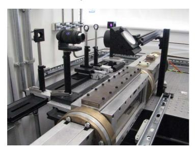
Fig. 53: Optical section of the flame tube along with the optical setup (final three mirrors, telescope and light sheet optics).
