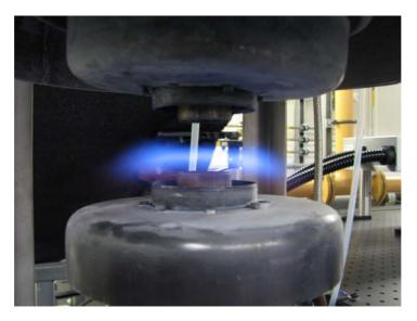
Fig. 34: Typical flame position of the reactants injected from the upper nozzle stabilised against the hot combustion products emerging from the lower nozzle.
