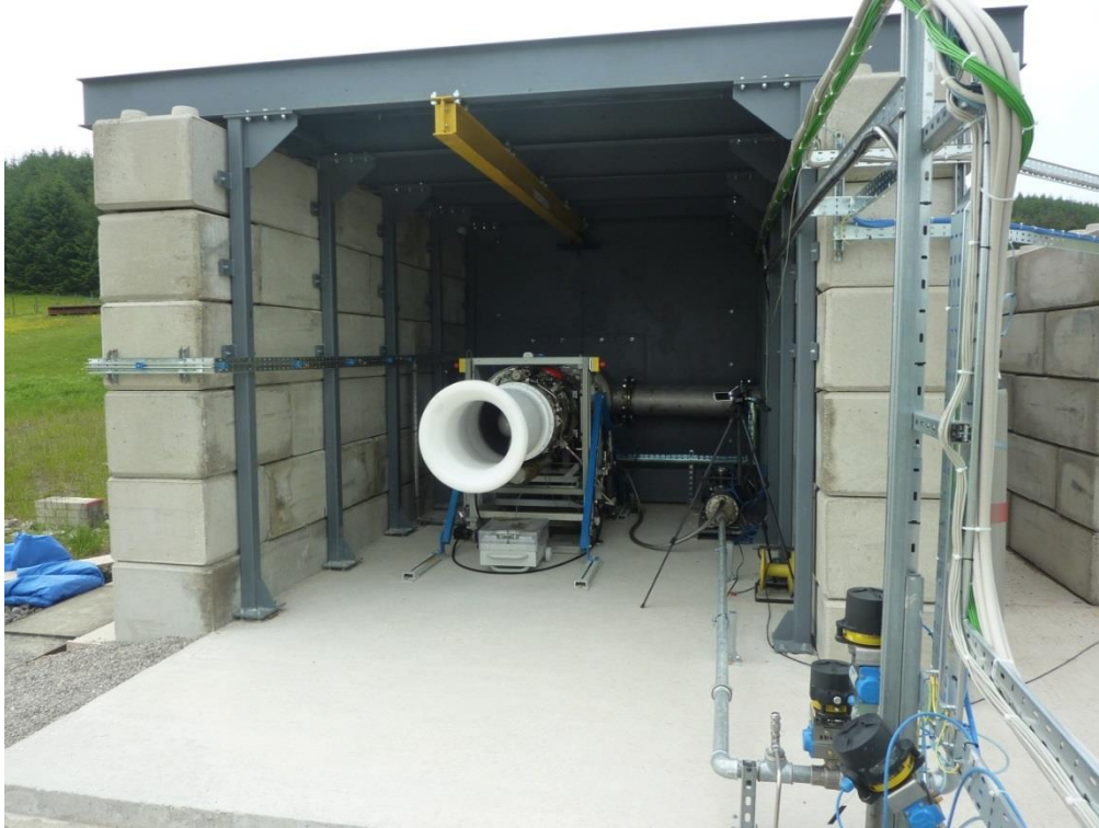
Figure 3: Viper engine in situ
