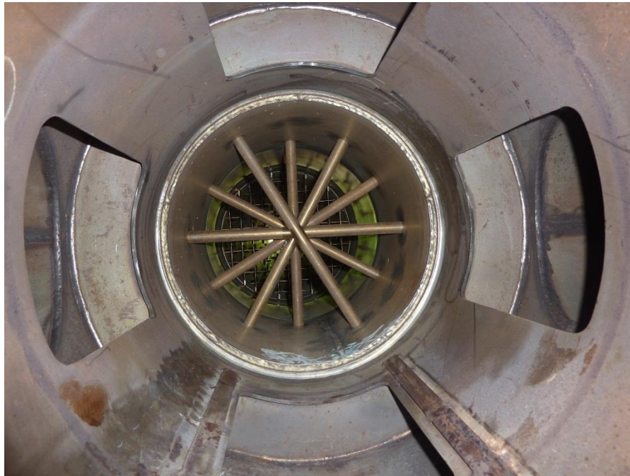
Figure 7: Gas diverter section
