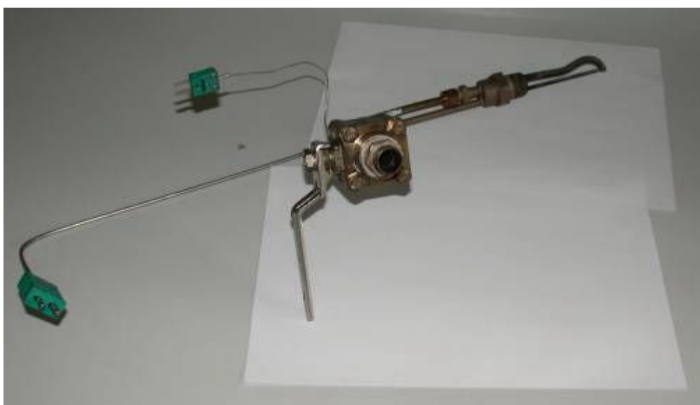
Figure 51. Special ECN tar and particulate sampling probe
