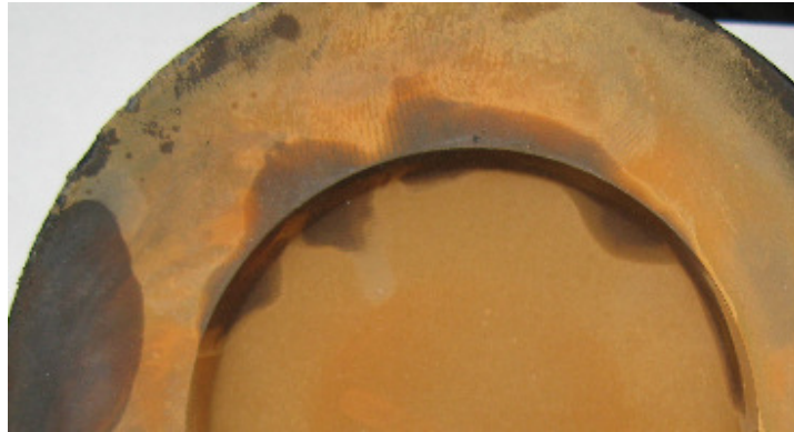
Figure 6 Rust on Piston Crown
