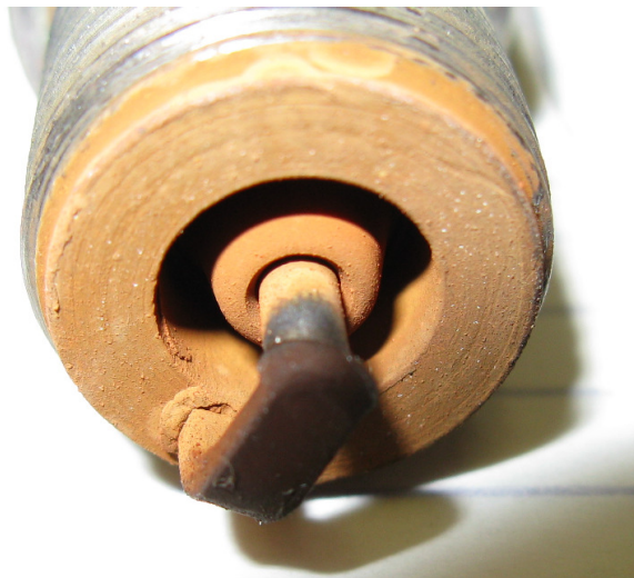
Figure 7 Rust on Spark Plug
