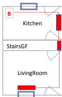
Figure A.7.2-2 Simplification of upstairs layout of Salford Energy House geometry to ease modelling
