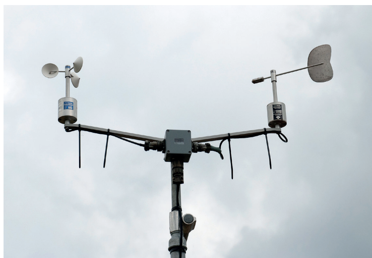
Figure 8. A cup anemometer with a wind vane on the adjoining arm of the mast. Measurements made by transducers in a heated sonic anemometer (not shown) can be combined to give an estimate of wind speed and direction in more extreme weather conditions. (© Crown Copyright Met Office 2018)
