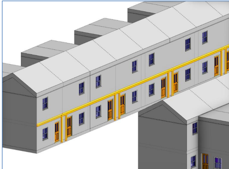
Figure 13: Typical arrangement of external wall pipe on front elevation about doorways with entry at ground floor level
