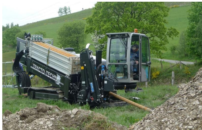
Figure 17: HDD equipment (Source: Tracto Technik)
