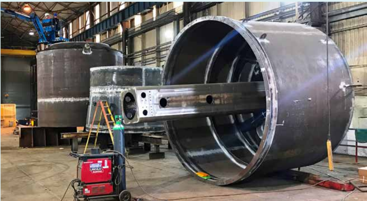
Archimedes Wave Swing being fabricated by Malin Group in Renfrewshire (Credit: AWS Ocean Energy)
