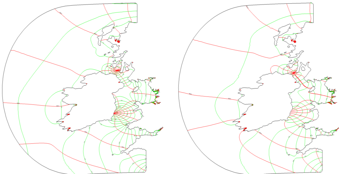
Figure 5.2.1: M_2 and S_2 co-tidal charts (amplitudes are plotted in green, with contour steps of 20cm and 10cm in left and right charts, respectively, and the phase is plotted in red, with contour steps of 20° in both charts).
