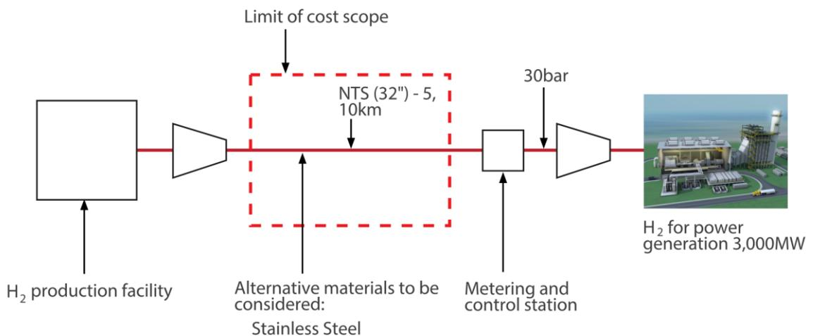
**Figure 7-1 Network schematic indicating scope boundary**
