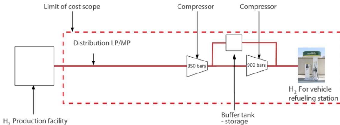
Figure 5-1 Network schematic indicating scope boundary
