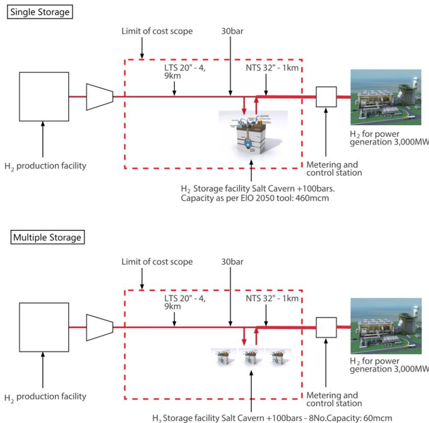
Figure 6-1 Network schematic indicating scope boundary
