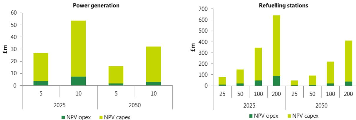
Figure 4-2 NPV (Capex and Opex) for the two scenarios
