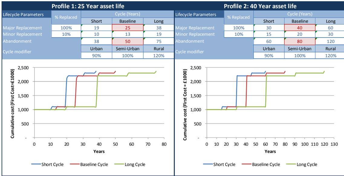
Figure 3-3 Lifecycle profiles in the ICC v1
