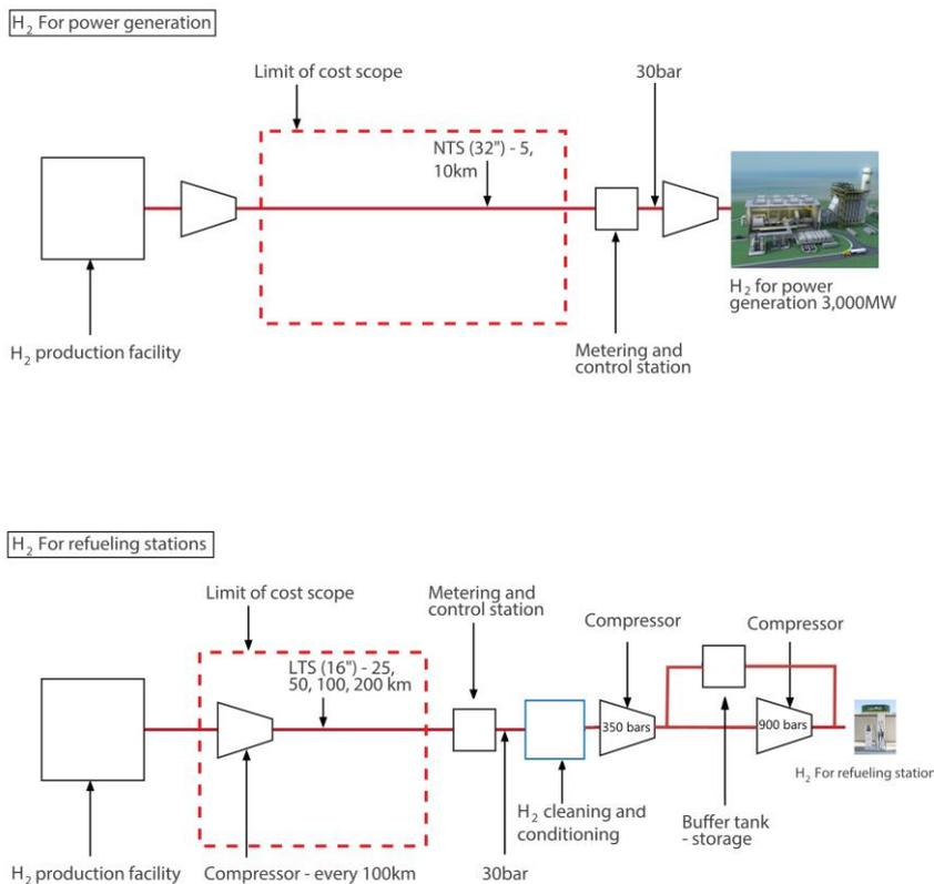
Figure 4-1 Network schematic indicating scope boundary
