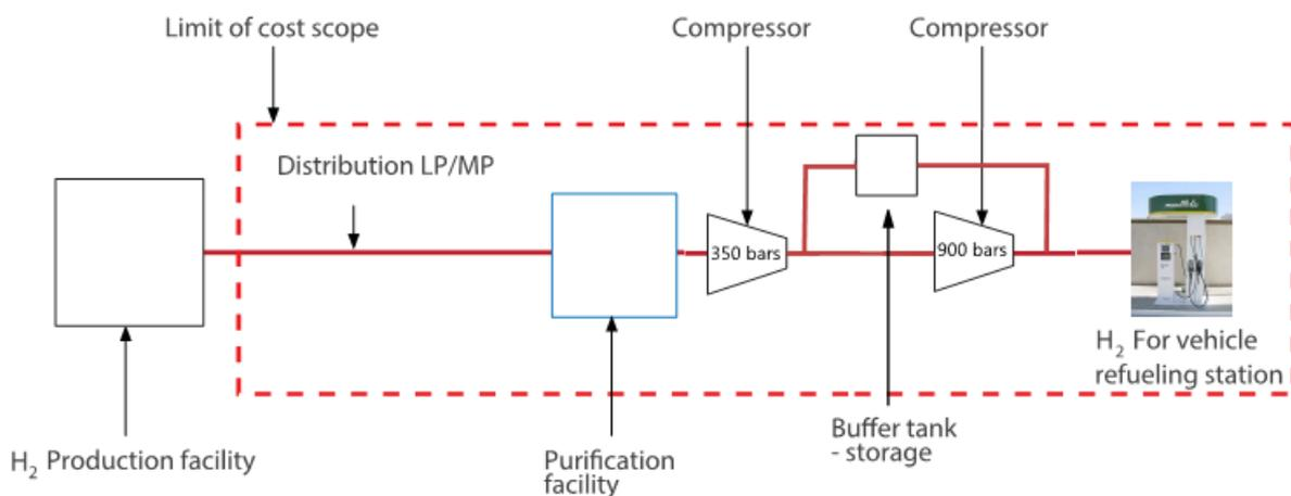
**Figure 8—1 Network schematic indicating scope boundary**
