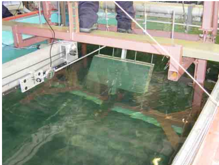
Figure 6 - Lancaster PTO system, attachment to collector
