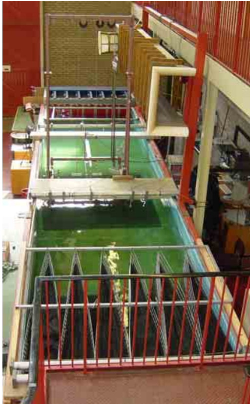
Figure 10 – Wave tank and corresponding schematic showing wave gauges (photograph courtesy Lancaster University Engineering Department)
