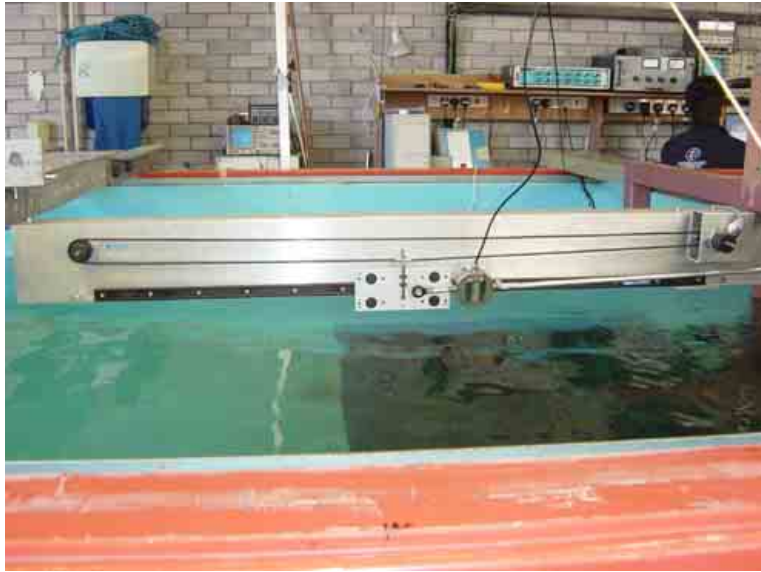
Figure 5 – Lancaster PTO system, toothed belt and slider
