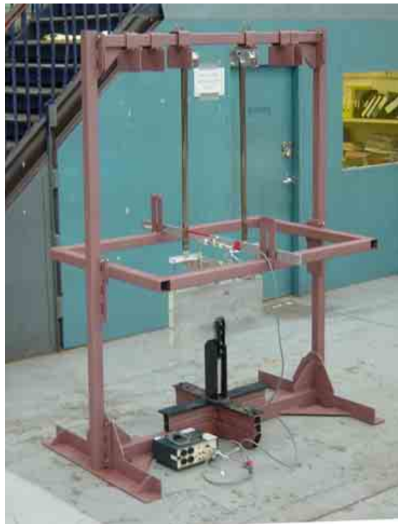
Figure 1: Test rig at Newcastle, comprising support frame, PTO and Restoring Force System
