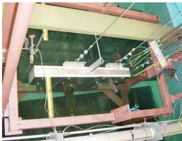
Figure 7 – Lancaster collector attachment to restoring force system
