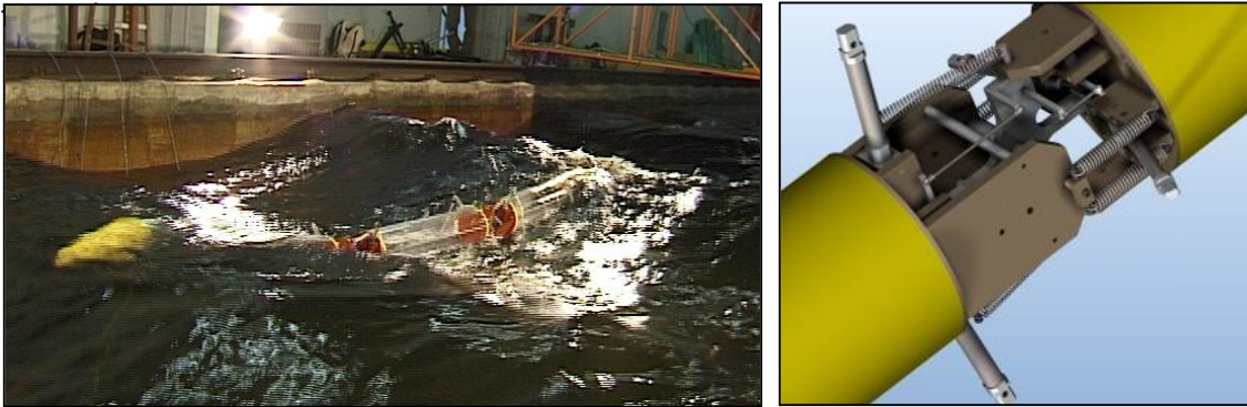
Figure B1.1 Mk1 20 th scale model under test and joint detail showing water dampers
