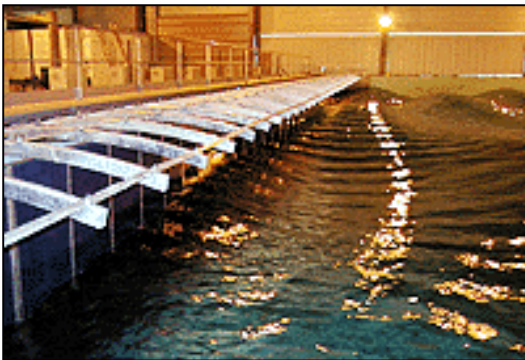
(Above) Wavemaker bank generating directional swell.
