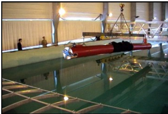
Figure A4.5 The two rear sections being craned into the main basin.
