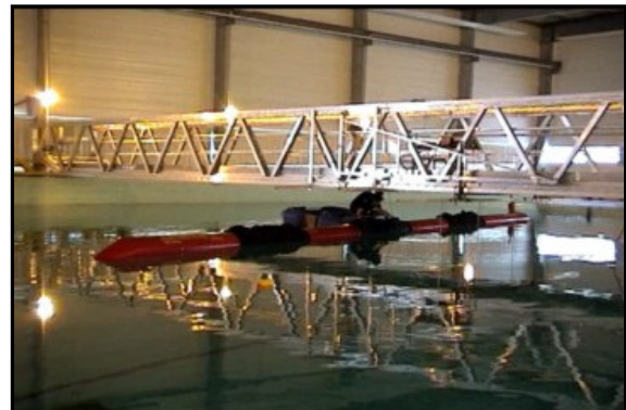
Figure A4.6 Joint of middle joint before model is wired to power and DAQ system. Note jackets around joints.
