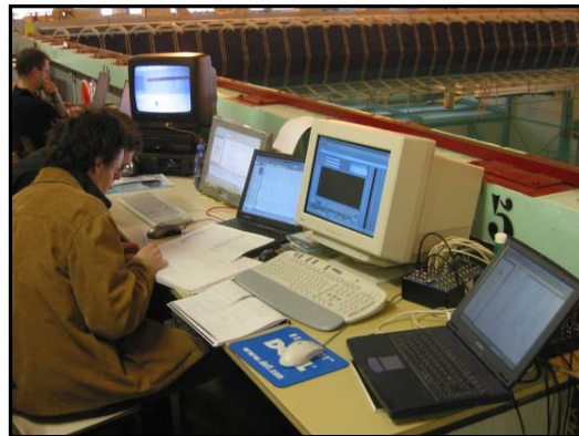
Figure A3.1. Control desk with video, control and DAQ systems
