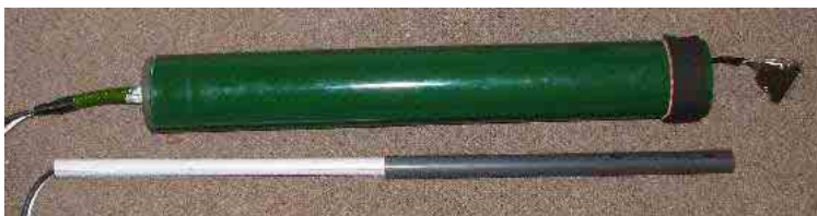
Figure 29: Barge POD, with data cable and lead to remote acoustic sensor (in foreground). Photo courtesy P. Fisher.
