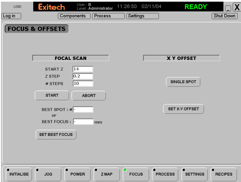
Screen for automated finding and setting of laser focus.
