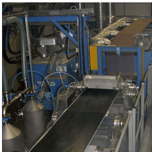
Small-scale dynamic nonwoven line for low cost substrate fabrications (courtesy of Technical Fibre Products Ltd)
