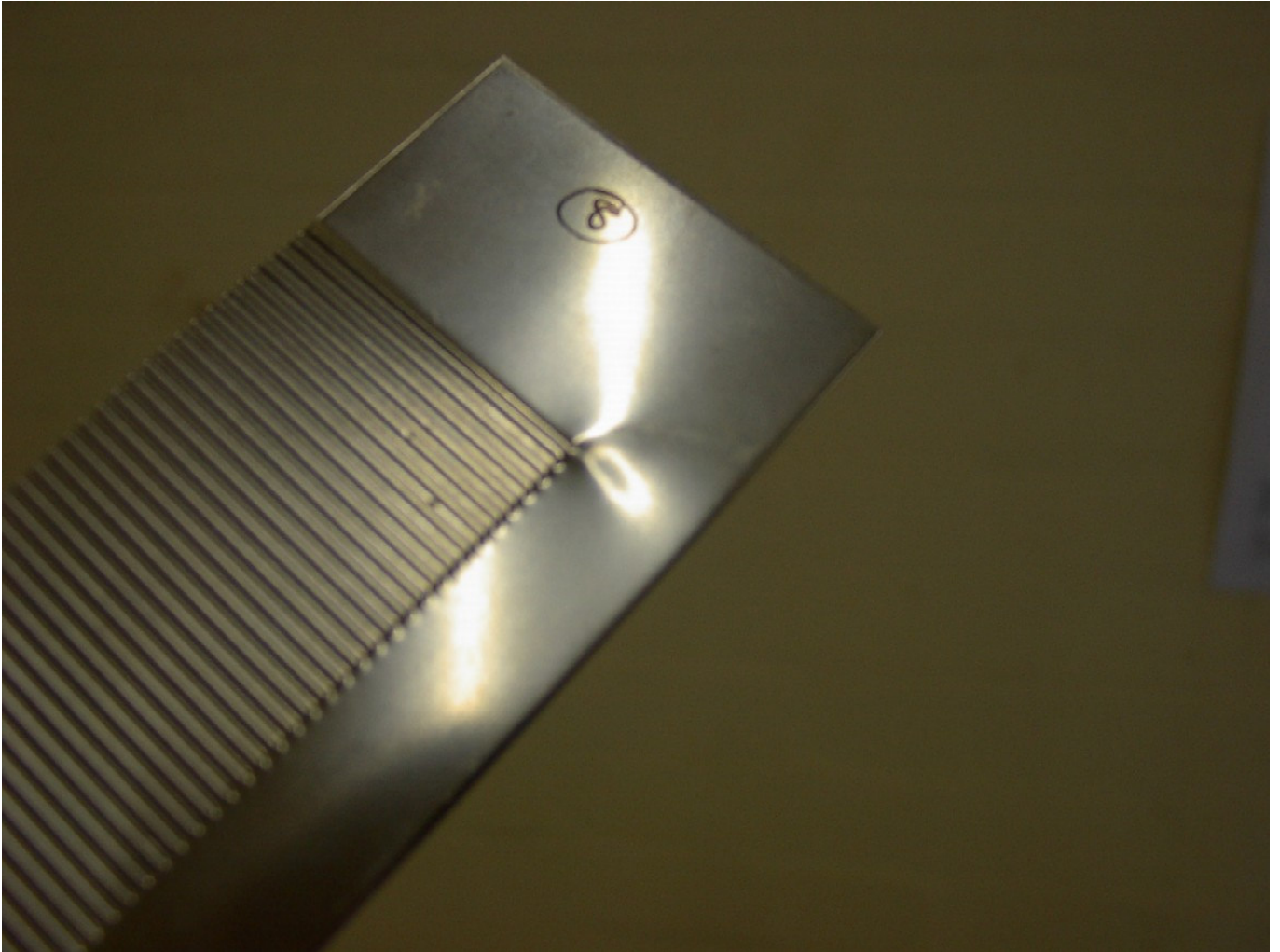
Figure 33. Prototype pressing showing "kink" feature.
