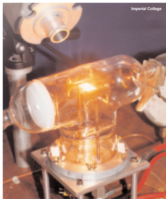
Figure 2. High Temperature Wire Mesh Reactor (courtesy of Imperial College London)
