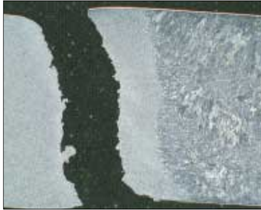
Type IV cracking in an E911 steel cross-weld creep test specimen
