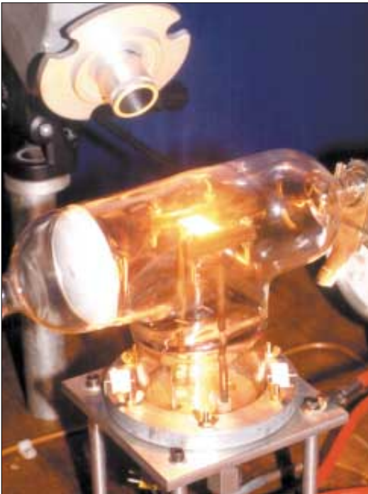
The Imperial College high temperature wire mesh apparatus (HTWM)
