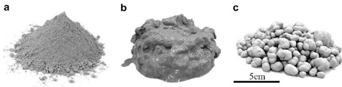
Figure 126 Raw materials: (a) paper ash, (b) quarry fines, and (c) pelletised product [Gunning, 2009]
