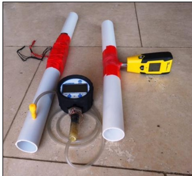
Figure 47: Fans, Anemometer and Pressure Gauge configured for use in a test loop
