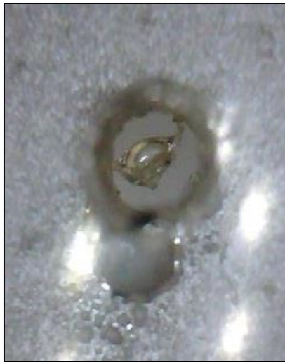
Figure 54: Bead of liquid seen across the leak in Test #1.2
