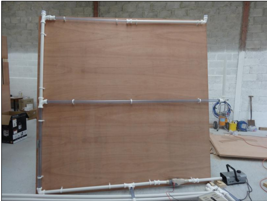
Figure 33: The first loop utilised elbows and tees
