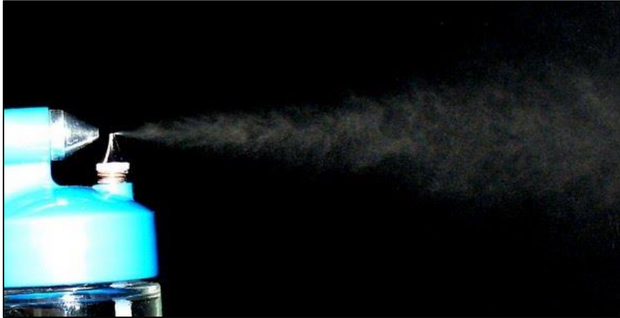
Figure 13: An atomised liquid aerosol generated from an artist's handheld airbrush
