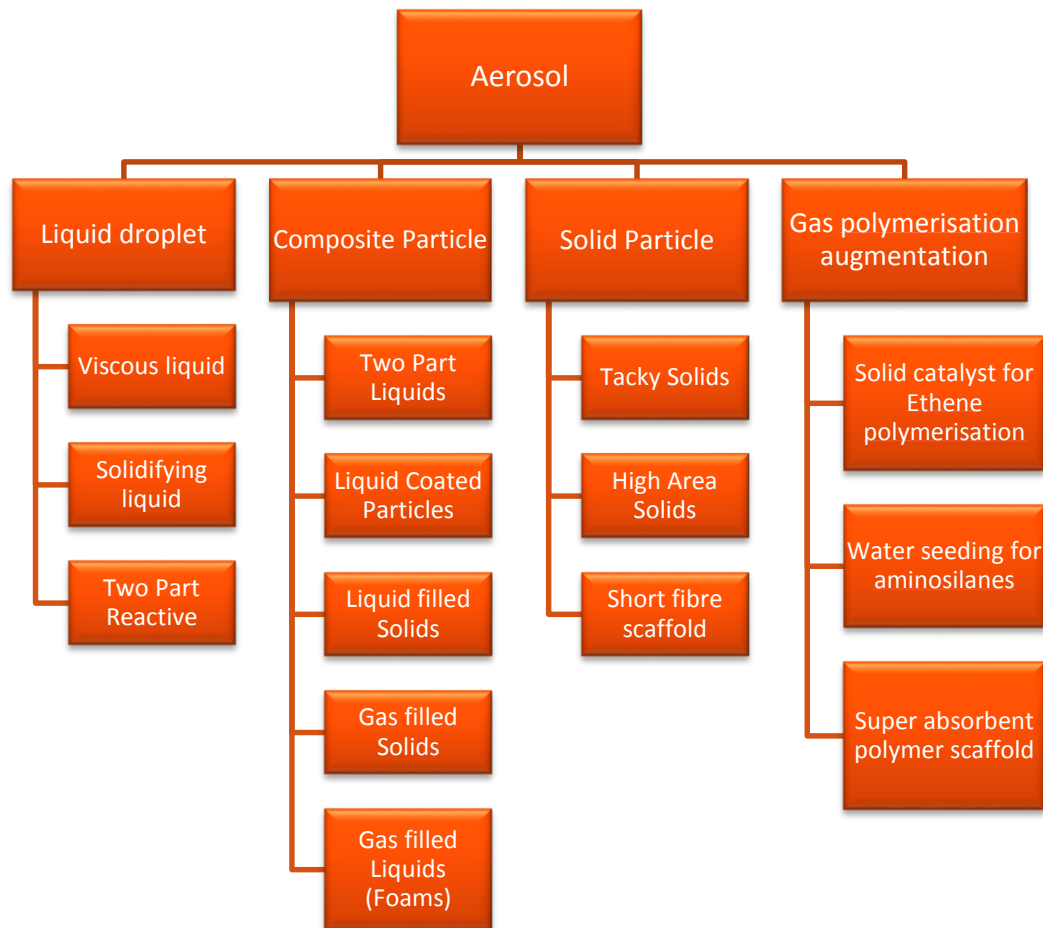
Figure 8: Initial classification hierarchy for the range of aerosol concepts to be considered
