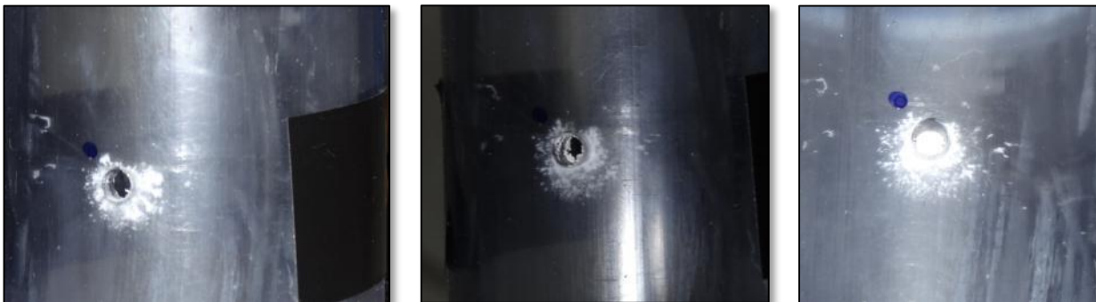
Figure 81: Sealing of the top relief hole in less than 30 minutes
