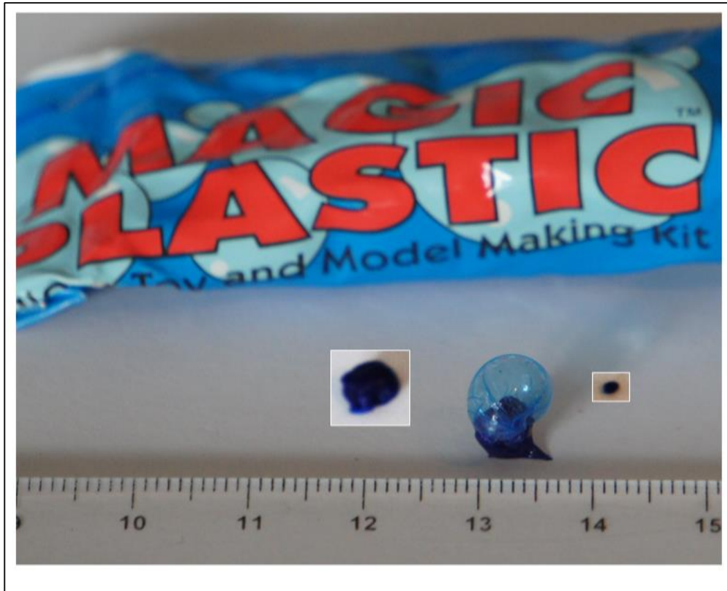
Figure 30: A polyvinyl acetate bubble with sprue. Inset are images on the same scale of the bubble and the sprue separated and rolled into spheres.
