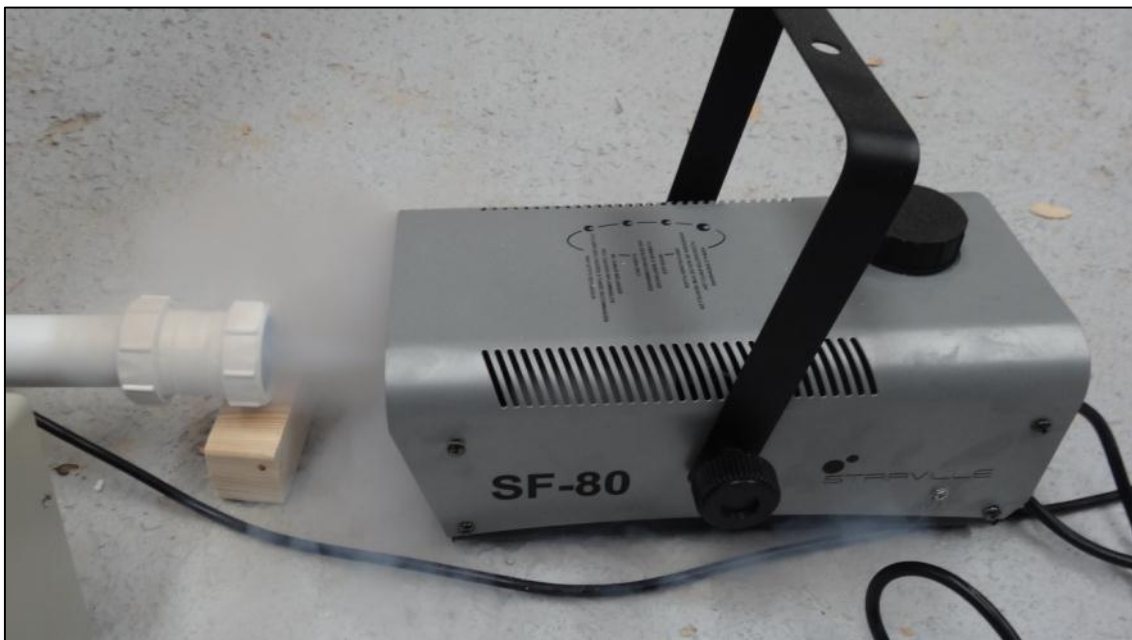
Figure 32: Fog Machine feeding into the loop
