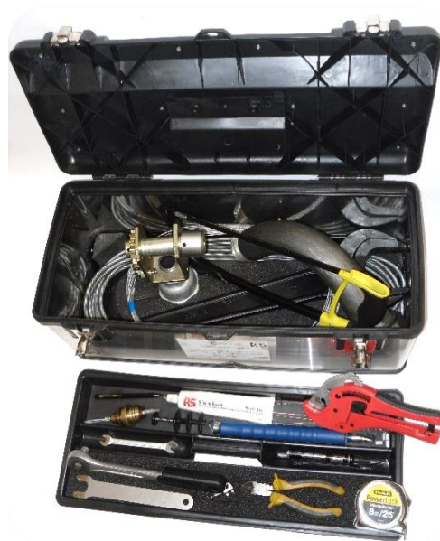
Figure 4: The 40mm Serviflex installation toolkit contained all the tooling identified by Radius Systems to complete the pipe installation.
