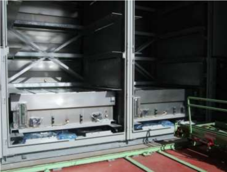
Figure 15 - Track allows quick repositioning of insertion tool
