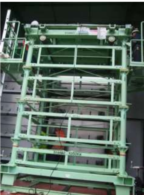
Figure 16 - Battery insertion tool at full height
