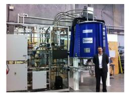
**Next Generation Post-Combustion (Gas):** Post-combustion CO<sub>2</sub> capture by solid adsorption. Novel technology based on rotating bed. Project led by Inventys (Canadian SME), supported by UK engineering. Canadian demo now proceeding with Husky
