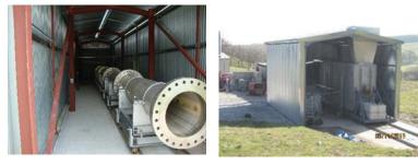
**High Hydrogen**: £4M investment to understand risks and identify safe operating conditions for turbines burning high concentration hydrogen mixtures
