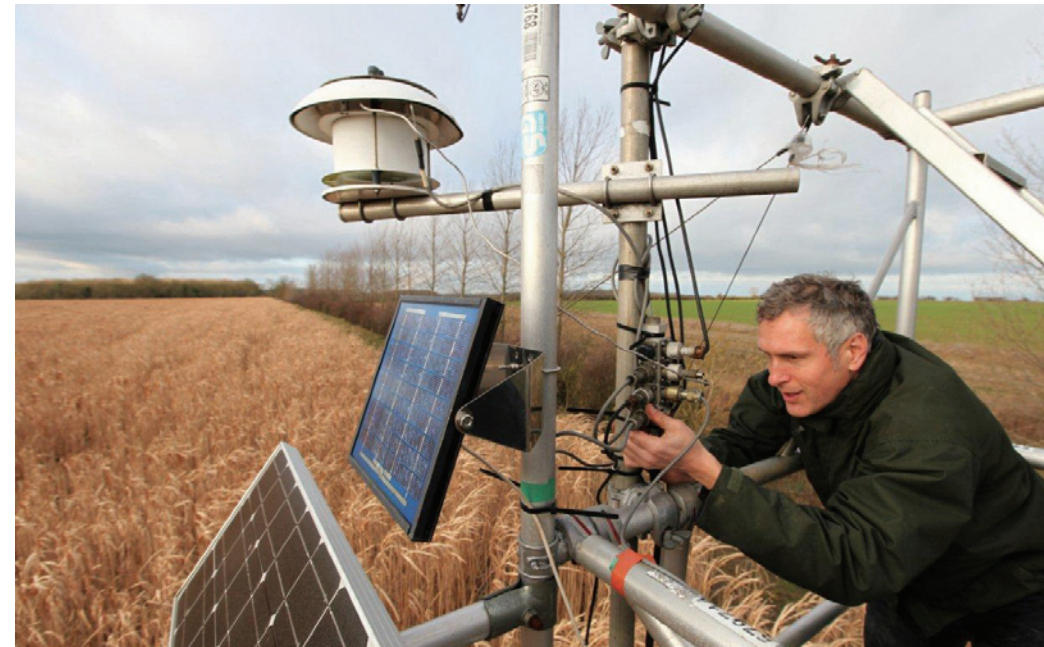
Measuring greenhouse gas fluxes from cultivated land under ETI's ELUM project
