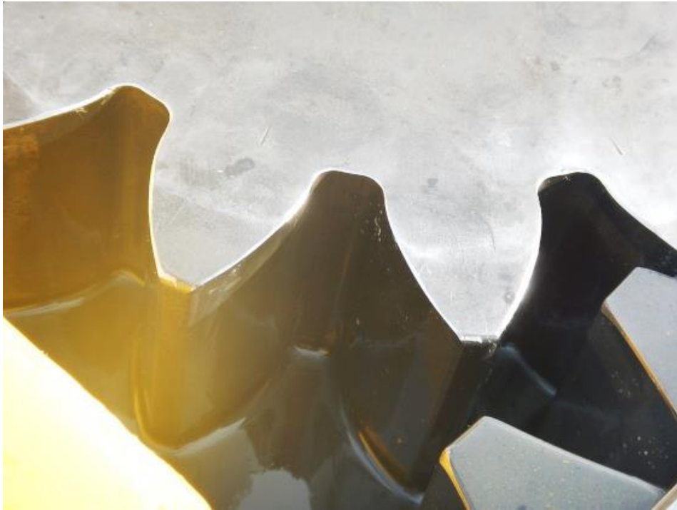
Figure 16 -Blade 3 pitch inspection - pinion close-up
