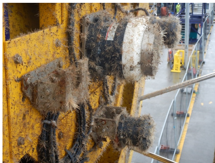
Figure 29 - Biofouling on the University of Edinburgh's thruster mounted instrumentation rack
