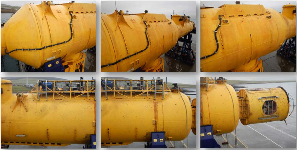
Figure 20: Nacelle condition after 145 days deployed at Fall of Warness
