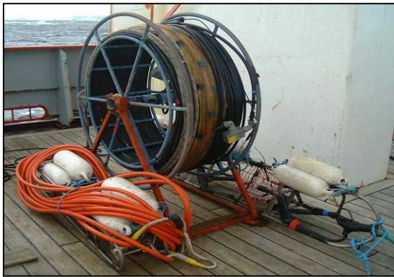
Figure 10-19: BGS tow fish (orange cable) hydrophones on reel (image courtesy British Geological Survey).
