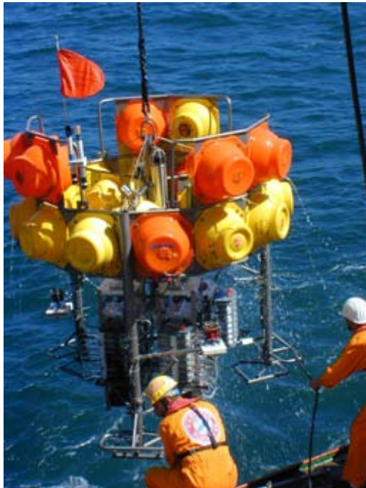
Figure 6-4: Photo of a Benthic Chamber Lander (image reproduced with permission of IFM-GEOMAR, ifm-geomar.de 2010).
